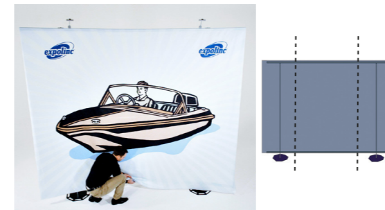
13 Press the plastic strip into the lower track of the profiles. This is easiest done from the back of the system. Make sure the graphic hangs straight.
